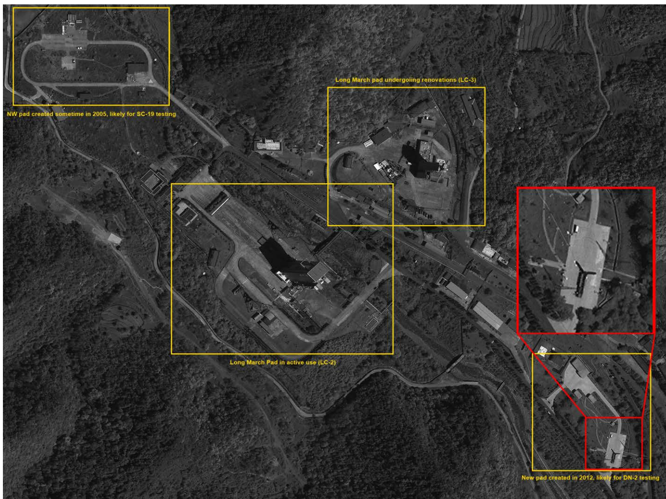
Imagery of Xichang from April 3, 2013, showing a TEL on the southeast pad. Image © 2013 DigitalGlobe. All rights reserved.
