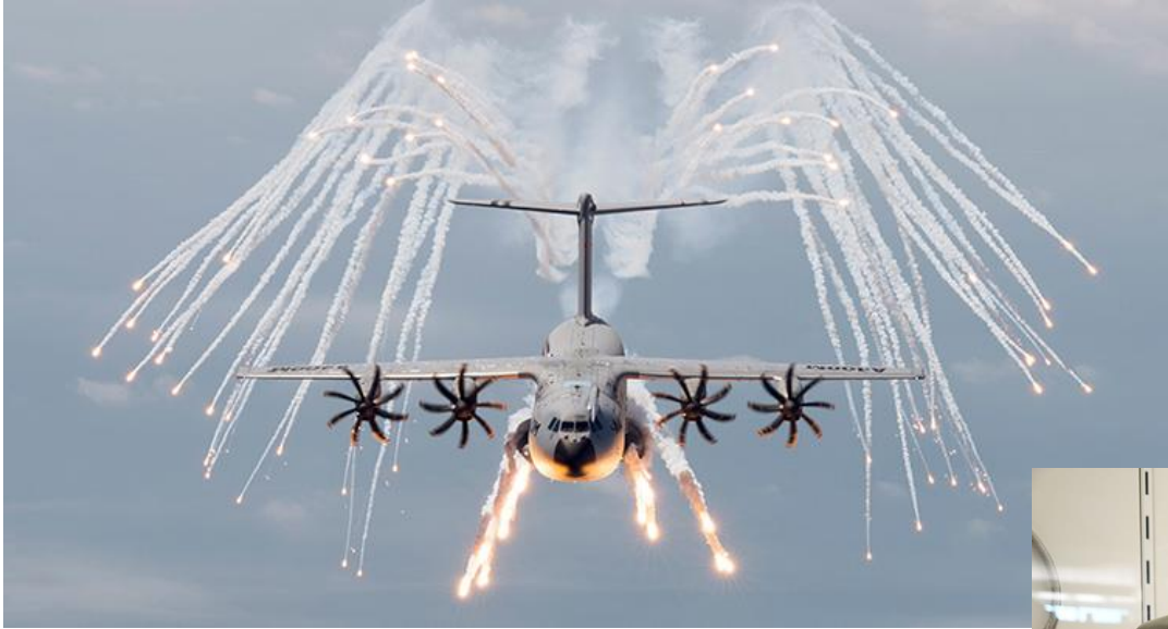
Flare and chaff anti-missile protections for transport aircraft Credit: Lacroix Defense
