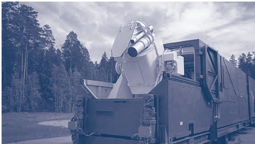
A Russian mobile laser system used to dazzle aerial and space reconnaissance assets.
