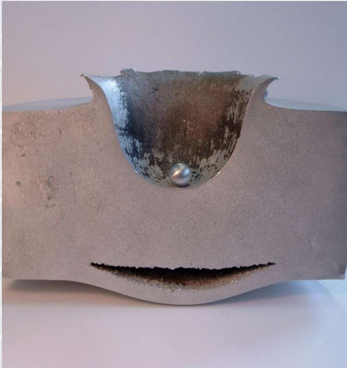
Impact crater created by a 13 mm object hitting an aluminum plate at 7 km/s (Credit: European Space Agency )
